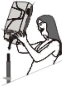
1. Attach an appropriate TV pin to the top end of the stand and fasten it with the handle at the side. Suitable TV pin: TV-35 TV-pin for speakers, No. 60000735.
